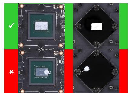
**EN** With the help of a plastic strip or similar spread a thin layer of thermal paste on the GPU. The layer should be less than a millimeter thick, otherwise the surrounding components may be contaminated unnecessarily.
