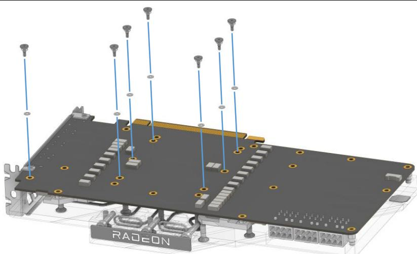
**EN** Place the graphics card on the prepared cooler. Fasten the card as shown with the 7 M2x5 screws with M2 washers. Hand-tighten the screws crosswise, one turn at a time.
