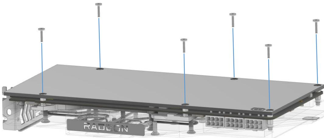
**EN** Put the backplate on and screw it together with the 6 M2x11 screws as shown.
