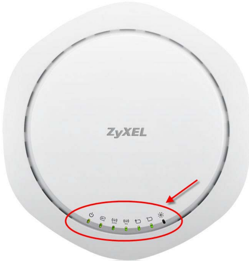
Figure 20 WAC6502D-E, WAC6502D-S, or WAC6503D-S LEDs
