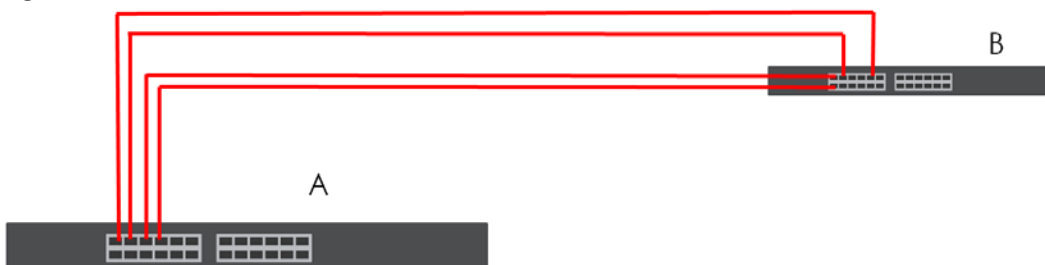
Figure 134 Trunking Example – Physical Connections
