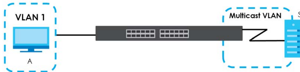
Figure 175 MVR Multicast Television Example
