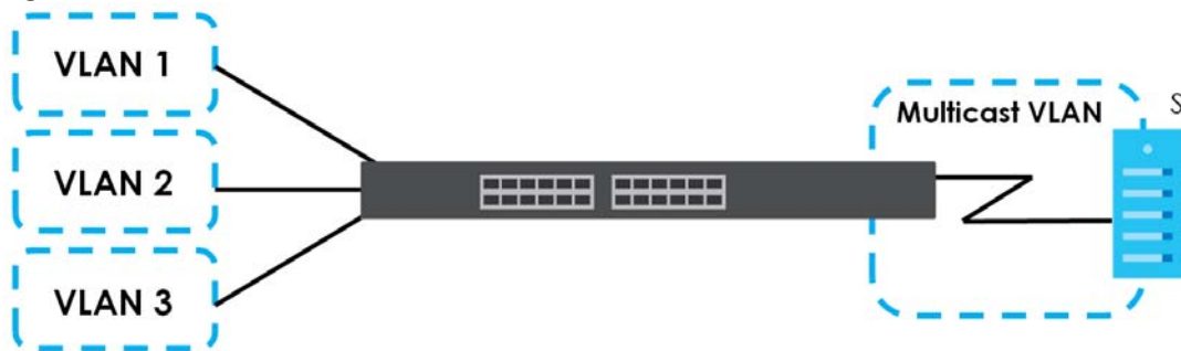
Figure 174 MVR Network Example
