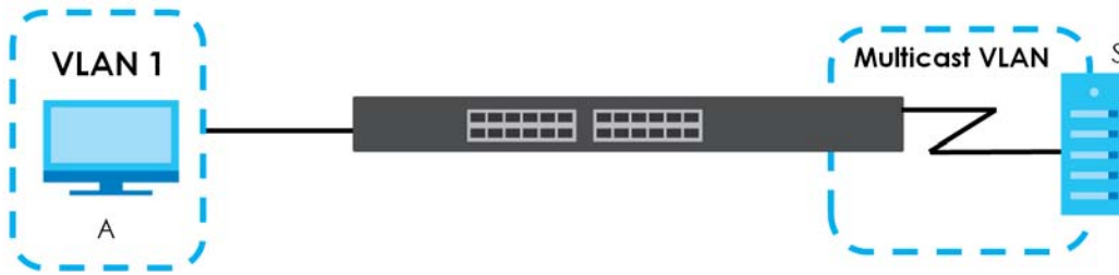
Figure 193 MVR Multicast Television Example
