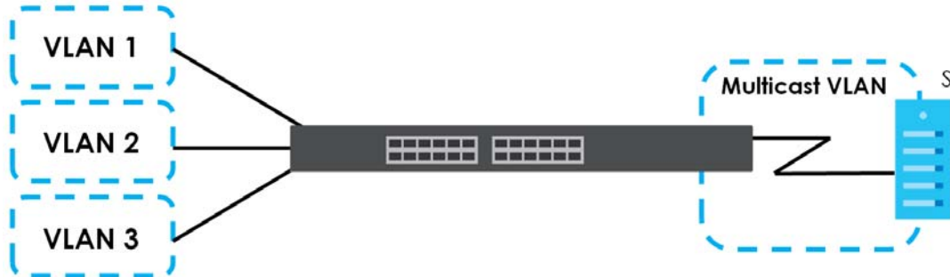
Figure 192 MVR Network Example
