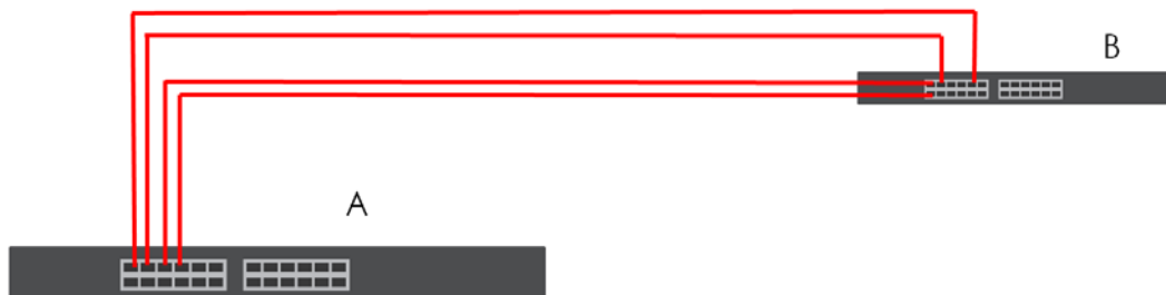
Figure 166 Trunking Example – Physical Connections
