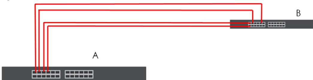
Figure 134 Trunking Example – Physical Connections
